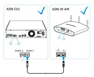
To optionally combine the antenna module with wired conference units, connect the antenna module just like a wired conference unit:
